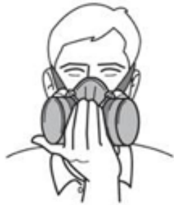
Positive pressure fit check
