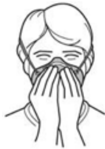
Seal check with a disposable respirator
