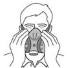
Negative pressure fit check
